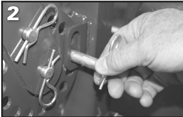
2 Unpin the adjustable tube from the hold down bracket as shown. Reinsert the pin in the hold down bracket.
