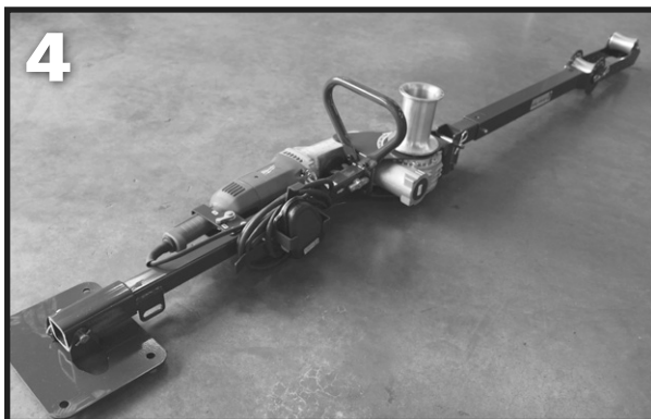
4 Cable puller shown unfolded and pinned.
