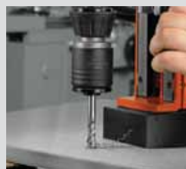
Tapping with fast change tapping chuck
