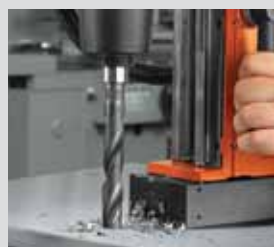
Twist drilling with chuck or MT 3 holder
