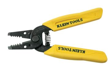
This compact, lightweight wire-stripping and cutting tool is designed to cut 10 - 18 AWG solid wire. The precision-ground stripping holes cleanly cut wire and aid in easy removal of insulation. A narrow nose helps this tool fit easily into tight places.
