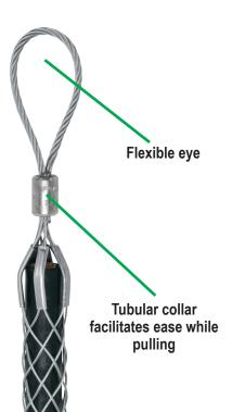
Pulling Grips are designed to serve as reusable tools for light industrial pulling of electrical cable and for underground and industrial plant wiring and re-wiring. These grips offer protection from abrasion and ease the cable through bends and rough surfaces. They also serve as a temporary splice, when replacing old cable with new, and to pull slack in new construction or maintenance operations.
