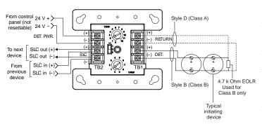
The FX-2WIRE can be set for Class B or Class A operation using the slide switch located on the front of the module.
