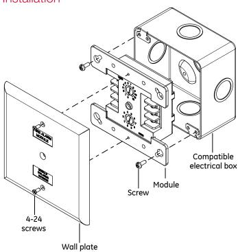
Mount in a North American 4 inch square  $\times$  2-1/2 in. (64 mm) deep 2 gang box or a standard 4 in. square box 1-1/2 in. (38 mm) deep.
