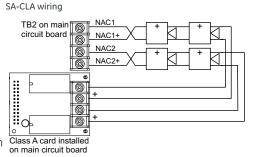
does not return to the SA-CLA card. The SA-CLA is compatible with FX-64 control panels only. FX-254 panels are Class A ready. The SA-CLA is installed directly to the control panel circuit board using its plastic standoffs and plug connection.
