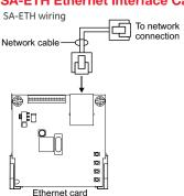
The SA-ETH card provides a standard 10/100 Base T Ethernet network connection for connecting to an intranet, a local network, or the Internet. The card can be used to download configuration programming from the FX-CU to the panel over the network.
