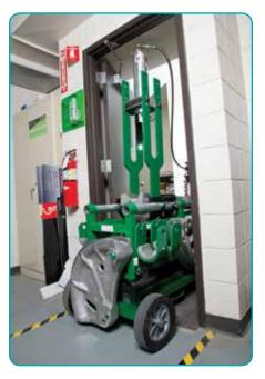
Forks of the 881 Bender Unit can fold down into the MBT for convenient transport or storage
