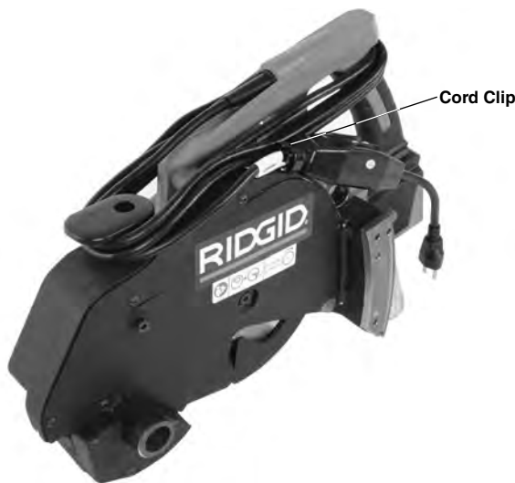
Figure 17 – Cord Wrapped for Transport
