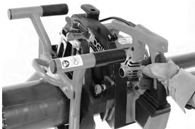
Figure 15 – PipeSaw Fully Plunged
