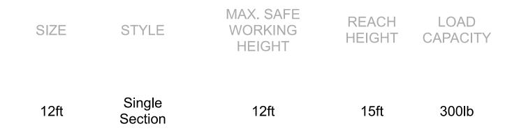
The D6212-1 Fiberglass One-Section 12ft Straight Ladders have non-conductive side rails and a duty rating of 300lb. Easy to transport and maneuver. Durable and long lasting. The Traction-Tred® D-rungs are slip-resistant. Durable rail shields and shoe brackets help to protect the rails from damage. The dual action feet pivot for use on hard or penetrable surfaces.
