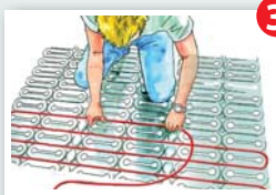
Install heating cable in grooves, pressing gently
