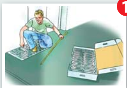
Lay out Reflect Plates
