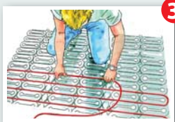
Install heating cable in grooves, pressing gently
