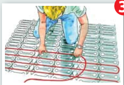
Install heating cable in grooves, pressing gently
