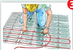
Install heating cable in grooves, pressing gently
