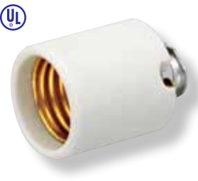
S70-560 Keyless medium base, porcelain socket, 1/8 IP hickey Packing: 72/Master, 6/Inner
