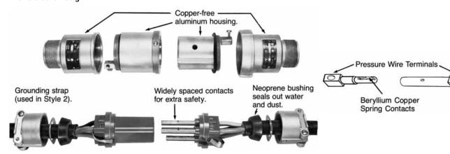
**Energized contacts** deeply recessed to reduce danger of accidental touching, minimize possibility of exposed arcs. Insulator quenches arcing, and is resistant to abnormal heat and to fire.
