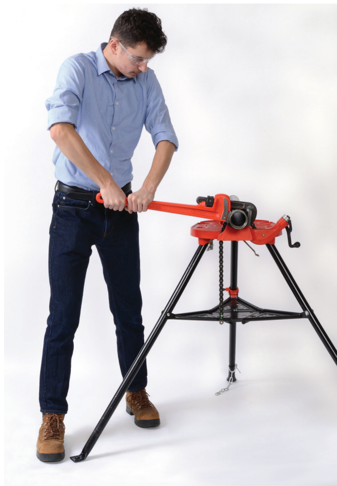
Figure 7 – A Proper Operating Position
