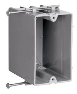
Single Gang, Deep Switch and Outlet Box with Captive Mounting Nails on Each End, Two Quick/Click Entries on Each End. It is a durable, impact-resistant thermoplastic boxand has innovative extras that cut installation time. Extra deep for dimmers, GFCI and thermostats, yet suitable for 2x4 construction. 100 pack.
