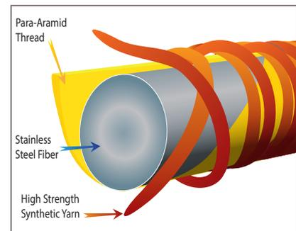
ANSI A6 cut protection liner includes steel fibers
