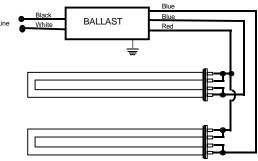
Note: For one lamp application, cap one blue lead, insulate to 600 volts
